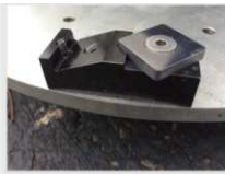
45° Mount for Sharp Cutting Point
