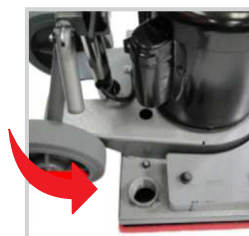
Milled Dust Control Access
