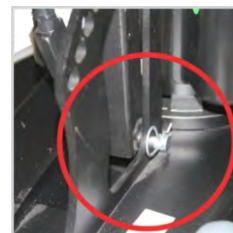
Remove the Handle Mounting Pin w/o Tools
