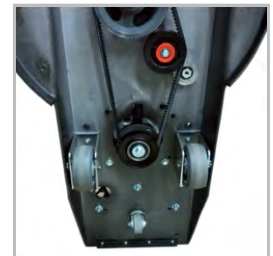
V-Belt Drives Pads at 2000 RPM
